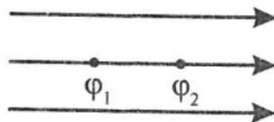
$$E = \frac{U}{\Delta d}; \quad [E] = \frac{H}{\text{Кл}} = \frac{B}{\text{м}}.$$
